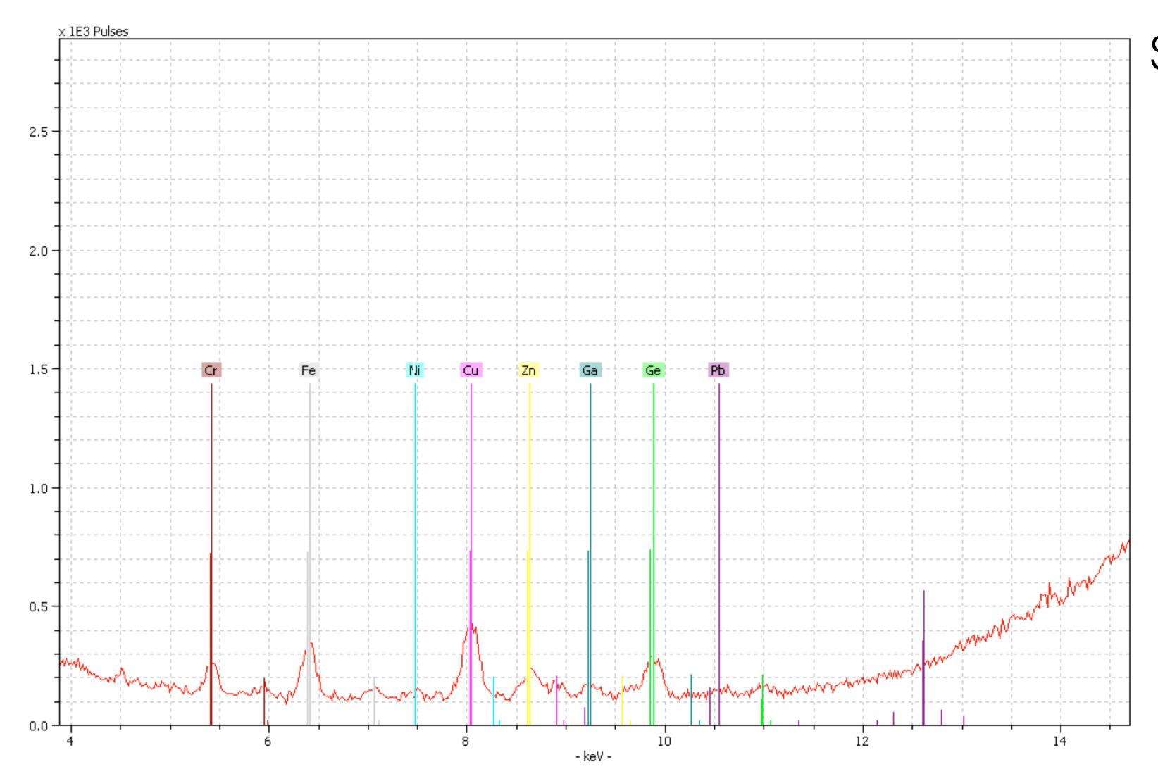
Some elements, like Topaz, have no unique elements as identifiers  $(Al_2SiO_4(F,OH)_2)$ . In this case, the proportions of elements can be used (twice as much Al relative to Si). Additionally, trace elements can be used to ID specific gems, such as the Germanium (Ge) and Galium (Ga) in this specimen.
