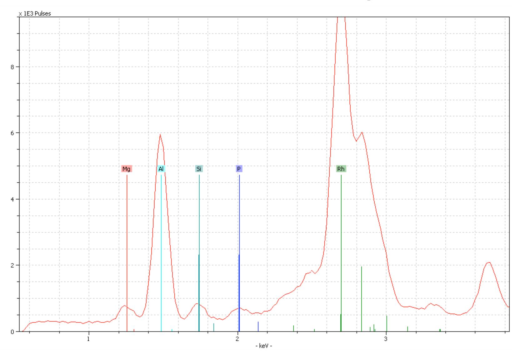
Spinel has the elemental concentration MgAl<sub>2</sub>O<sub>4</sub>.We would expect to see both Aluminum (Al) and Magnesium (Mg). Here, we see both in an authentic piece.
